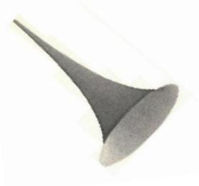
The surface obtained by rotating the tractrix around the y-axis is known as a *tractroid* (refer to the diagram on the right) and provides a model of a *pseudo-sphere* (a surface of constant negative curvature).
