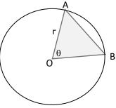
It is clearly wrong to apply this formula to obtain the 'distance' between A and B when the angle  $\theta$  is large. For example, if A and B are points chosen to be diametrically opposite, then the straight line 'distance' AB would be 2r, whereas the 'distance' measured along the circular arc using the formula above would instead be  $\pi r - an$  error of about 57%!
