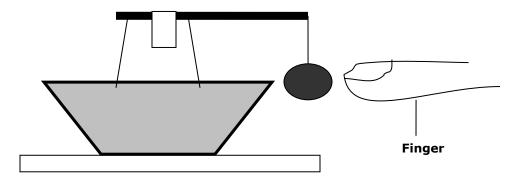
5) **Making a simple electroscope:** use a metal drinks can and tape it to an insulating base such as a styrofoam cup. Cut a strip of aluminum foil and fold it in half so as to be able to hang the foil through the tab of the can as shown below.
