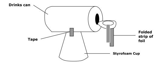
Now, repeatedly use your electrophorous to charge up the drinks can and observe carefully what happens to the two leaves of the aluminum strip as you repeat the process. Distinguish between the situations in which you bring the charged electrophorous a) close to the can (but being careful not to allow them to touch; and b) the electrophorous and can are in contact.
